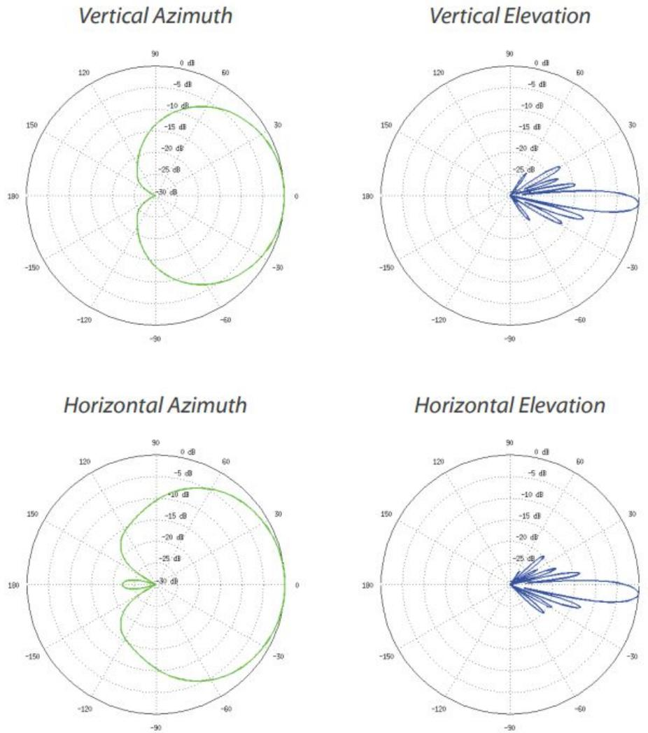
**Figure 3: 5.8 GHz Antenna Radiation Patterns**
